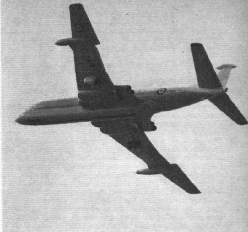
A view of the Nimrod which will become increasingly common over the years, especially at St Mawgan and Kinloss. The large bomb-bay doors are slightly open, and the dorsal fin and ECM fairing are distinctive
