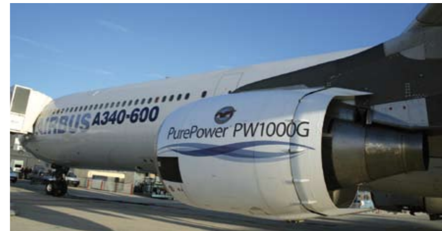
Airbus is flight-testing the GTF before deciding whether to adopt it for a narrowbody application
