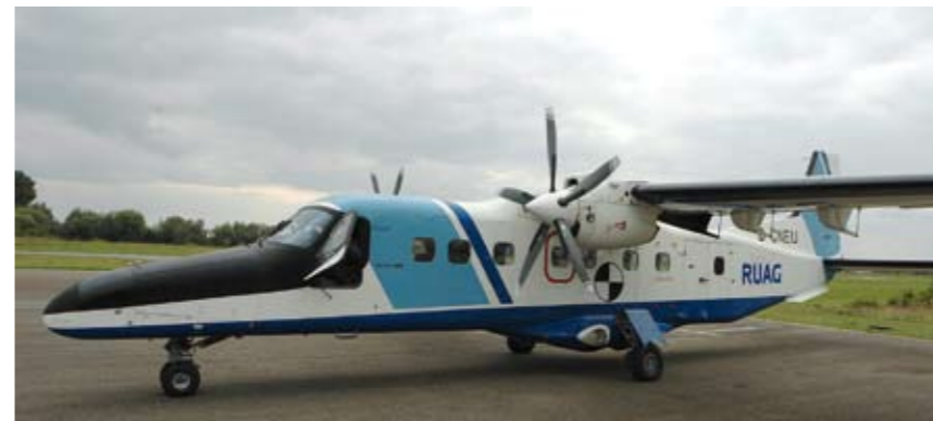
Ruag's relaunched Dornier 228 is equipped with MT-Propeller's five-bladed props
