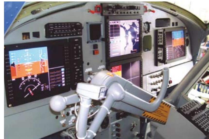
Viking Air's upgraded Twin Otter 400 features a new Honeywell cockpit
