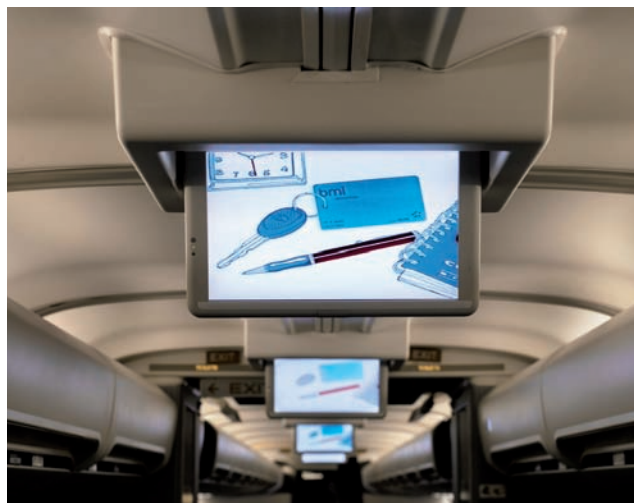
Line up for Airline Service's high-def 17.5in retractable screens.
