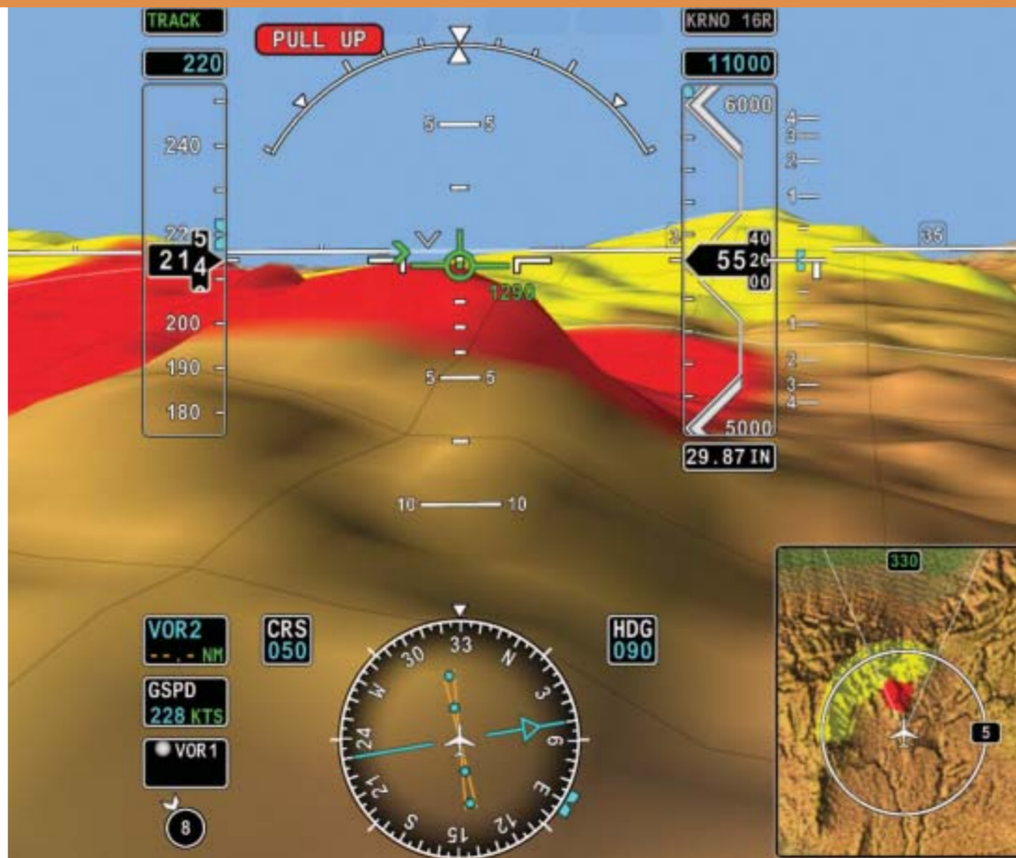
Above: Honeywell's EGPWS alert becomes even more apparent when shown on the SVS as shown on this approach. Right: CMC Electronics' SureSight I-Series Enhanced Vision System sensor is standard gear aboard the Global Express XRS and an option on the Global 5000, pictured here
