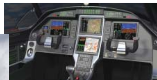
The legacy PC12/47 - there are no exterior changes. The BMW Designworks USA redesigned the cockpit to increase functionality and comfort featuring Honeywell's Primus Apex integrated avionics.
