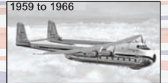
1959 to 1966 Manufacturer: AW Type: Argosy Seats: 65/freight Description: Freighter Number built: 17 (+56 military versions)
