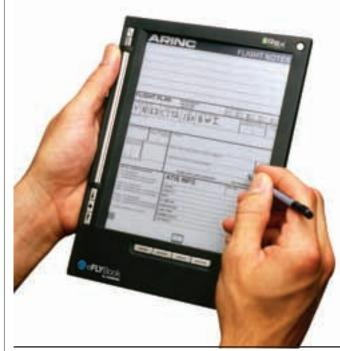
Arinc (stand 758) has joined the battle against paper in the cockpit, launching a tablet PC-based "mini-electronic flight bag" called eFlyBook that can be used to view en-route charts, approach plates and other flight documents in all light conditions.
