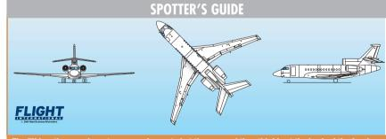
The 7X has three engines; two are pod mounted at the rear and then third is at the back of the fuselage with its air intake in front of the tail and on top of the fuselage. The wings are swept with winglets, the horizontal stabilisers are swept and mid-mounted.
