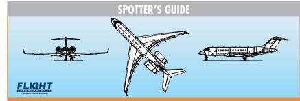
With 15 windows – Two more than the original Global Express – on each side of the cabin it clearly differentiates the XRS from the Global 5000 (with 10) and the Global Express (13). The outline of the Global Express is familiar with effectively a CRJ fuselage mated to a low swept supercritical wing with winglets. It also features a swept T-tail with swept anhedral tailplane.
