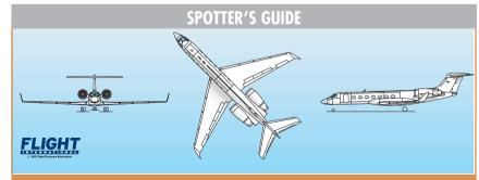
This aircraft differs externally from the legacy Gulfstream V by a seventh passenger window on the left side of the aircraft (as opposed to six on the left and either six or seven on the right). It features a low swept wing with winglets, twin Rolls-Royce Deutschland BR710 turbofan engines mounted on the fuselage ahead of a swept T-tail and swept tailplane.
