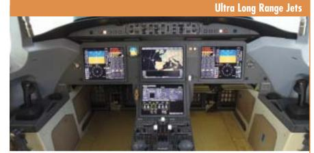
**THE** <sup>7X</sup> is the newest tri-jet member to join the Dassault Falcon family. It features Fly-By-Wire controls and was designed in a completely virtual environment. Originally the specifications called for a 5,700nm (10,556km) range. However, following customer feedback Dassault installed a new fuel tank forward of the wing centre section, increasing fuel capacity by 1,760lbs (800kg) and fitted drag reducing winglets.
