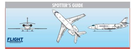
The Falcon 2000 is a direct descendent of the Falcon 900 – but without the third engine. The P&WC 308C engines are mounted on the sides of the rear fuselage. There are only nine windows compared to the F900's 12, but there is a similar tall swept tail fin and mid mounted swept tailplane.
