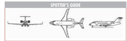
Although only two inches (5cm) bigger than the 604 windows, the Challenger 605 windows look much larger. A good identifier for the Challengers is the arced mounting for the engines. The low swept wing with winglets give this aircraft a fine look. The new Challenger tailcone has an angular finish, not flush like that of the 604.
