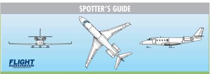
Despite having a larger cabin than the old G100/Astra SPX Gulfstream have reduced the number of windows by one – there are five on the left-hand side and six on the right-hand side. Originally it had six rectangular windows but these have given way to the distinct "oval" Gulfstream look. The low swept wing with winglets and the swept tailfin with low mounted swept tailplane remain very similar to the G100.
