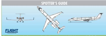
The aircraft has a circular cross-section fuselage, rear-mounted high by-pass ratio Rolls-Royce engines, low-mounted swept wings with blended winglets and a T-tail with swept tailplane. The wings are of two-spar wing design, with a third spar to support the landing gear. The Legacy has integral wing tanks, belly tanks and aft fuel tanks in extended fairings on the underwing.
