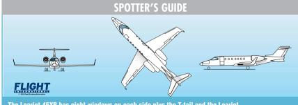
The Learjet 45XR has eight windows on each side plus the T-tail and the Learjet winglets makes it easily recognisable on the ramp.
