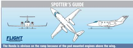
The Honda is obvious on the ramp because of the pod mounted engines above the A T-tail and large winglets will also help to identify this jet.
