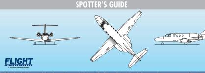
A CitationJet forward fuselage is mounted to a T-tail configured tailplane and a new supercritical laminar flow wing. The Williams FJ44 turbofans (with paddle thrust reversers) are mounted aft. A useful differentiator against other Citations is that CJ1 and CJ1+ have four windows.
