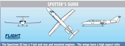
(the aspect ratio refers to the total span of a wing divided by the mean chord – where the chord is the length from the leading edge to the trailing edge) un-swept wing with winglets. Essentially high aspect ratio wings tend to be long and narrow, and low aspect ratios short and stubby. The 33 features five windows on each side and the cabin door is on the port side.
