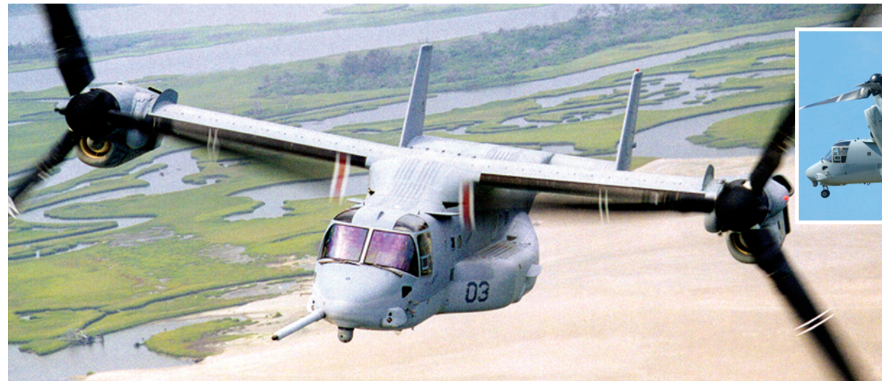
Easy up! The V22 tilts its rotors to suit mission.
