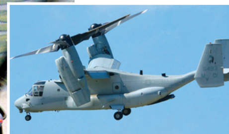
Easy up! The V22 tilts its rotors to suit mission.
