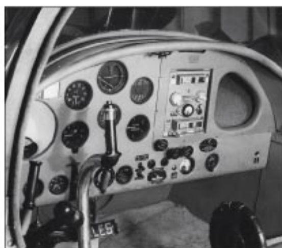
LEFT The Gemini had a neat and business-like instrument panel with a Plessey VHF transceiver installed in the glove pocket, leaving ample space for other uses.
